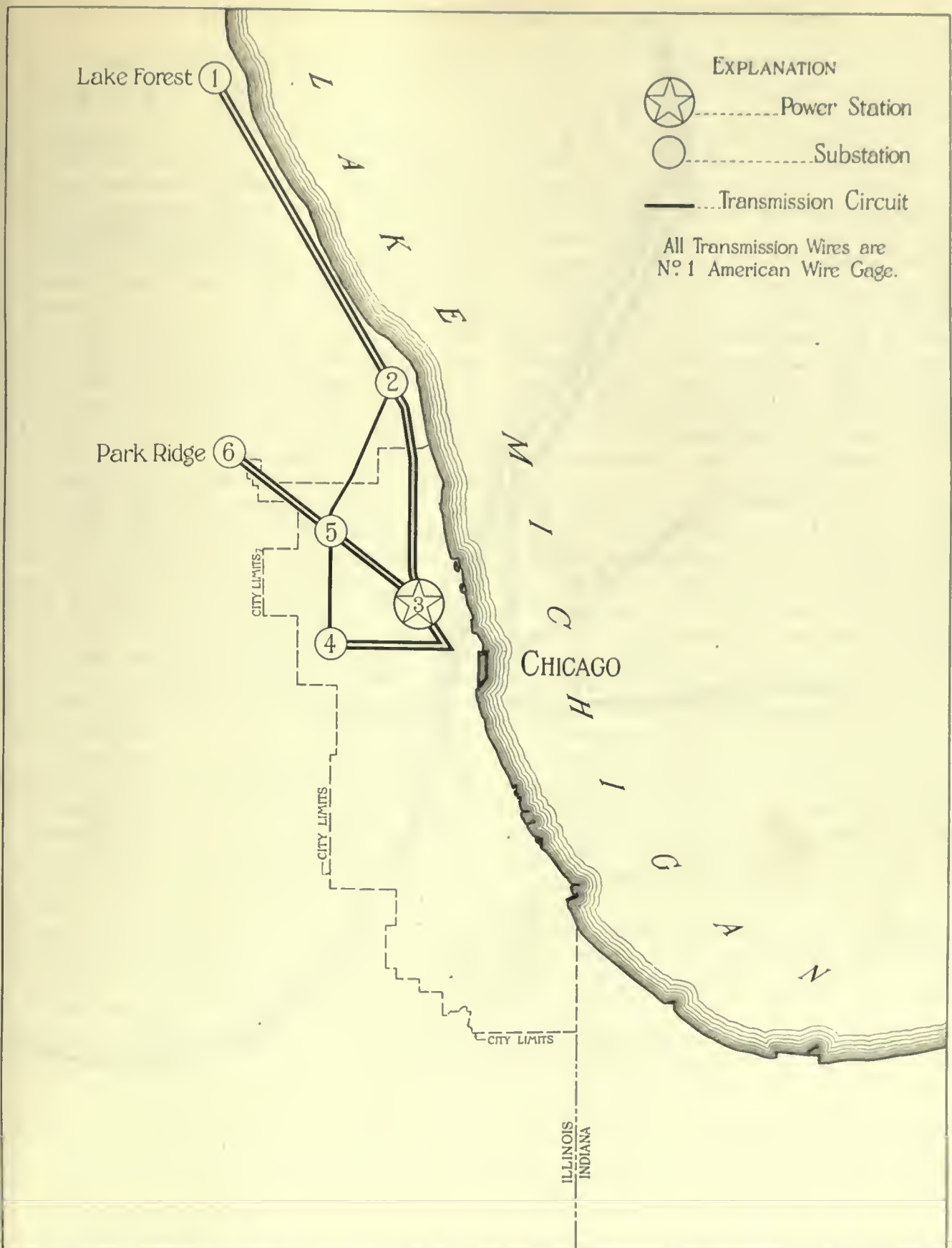
FIG. 682. TRANSMISSION CIRCUITS FOR THE 2,400-VOLT D. C. SYSTEM CHICAGO & NORTH WESTERN RAILWAY
